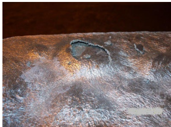
Figure 6: Surface Shrinkage Voids
