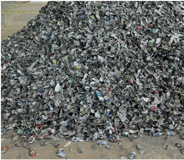
Figure 1: Excessive Painted Scrap in 3XXX Shreds
